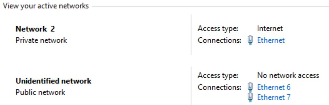
In this case, the new interfaces are Ethernet 6 and Ethernet 7. These will be the interfaces seen in Wireshark.
